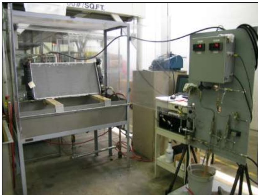
Figure 3: Radiator assembly burst pressure test setup at Delphi Technical Centre, Lockport, NY
