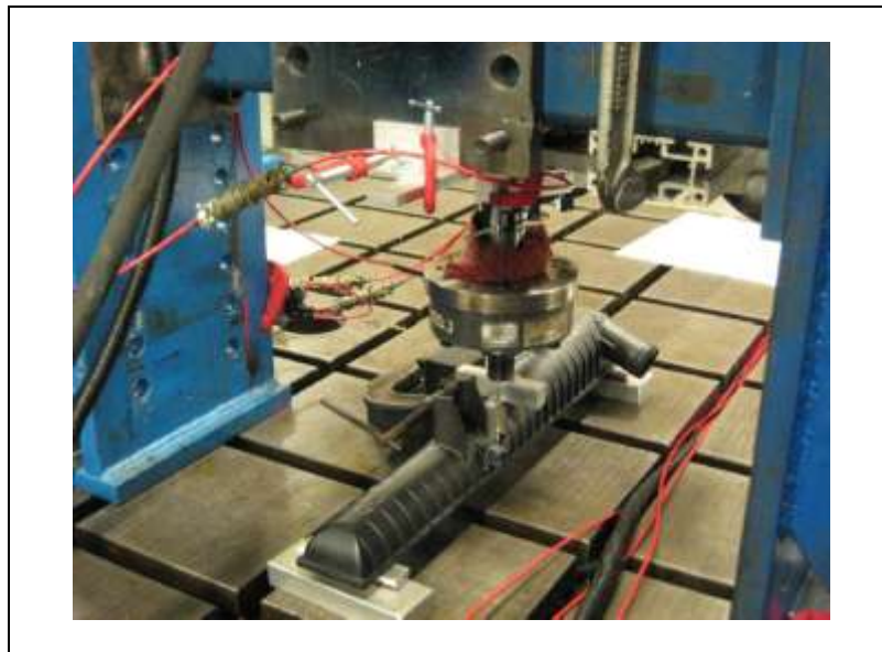
Figure 13: Experimental setup for three-point Bend test on radiator end tank
