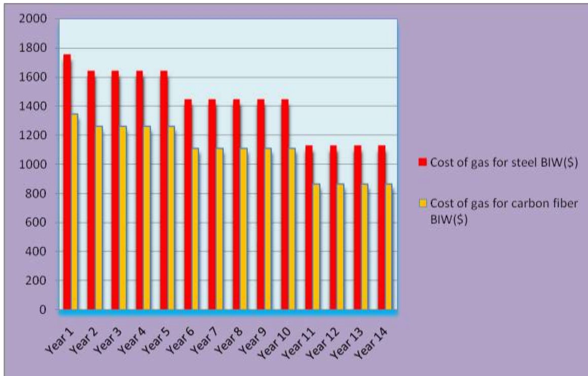
Figure 1: Use cost for carbon fiber BIW Vs steel BIW
