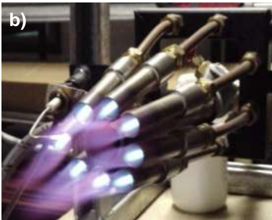
a) Figure 1: (a) Propane-fuelled burner. (b) Outer shroud removed to show ignited burners. (c) Tip of burner indicating how hot air stream converges with powder delivery stream.
