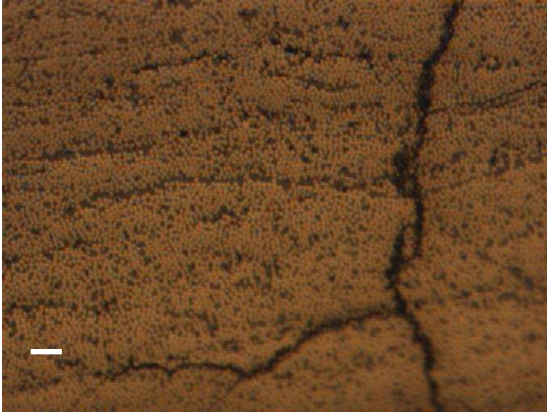
Figure 7. Typical microcracking of Epoxy sample after 20 cycle. Bar is 50 \mu\text{m} .
