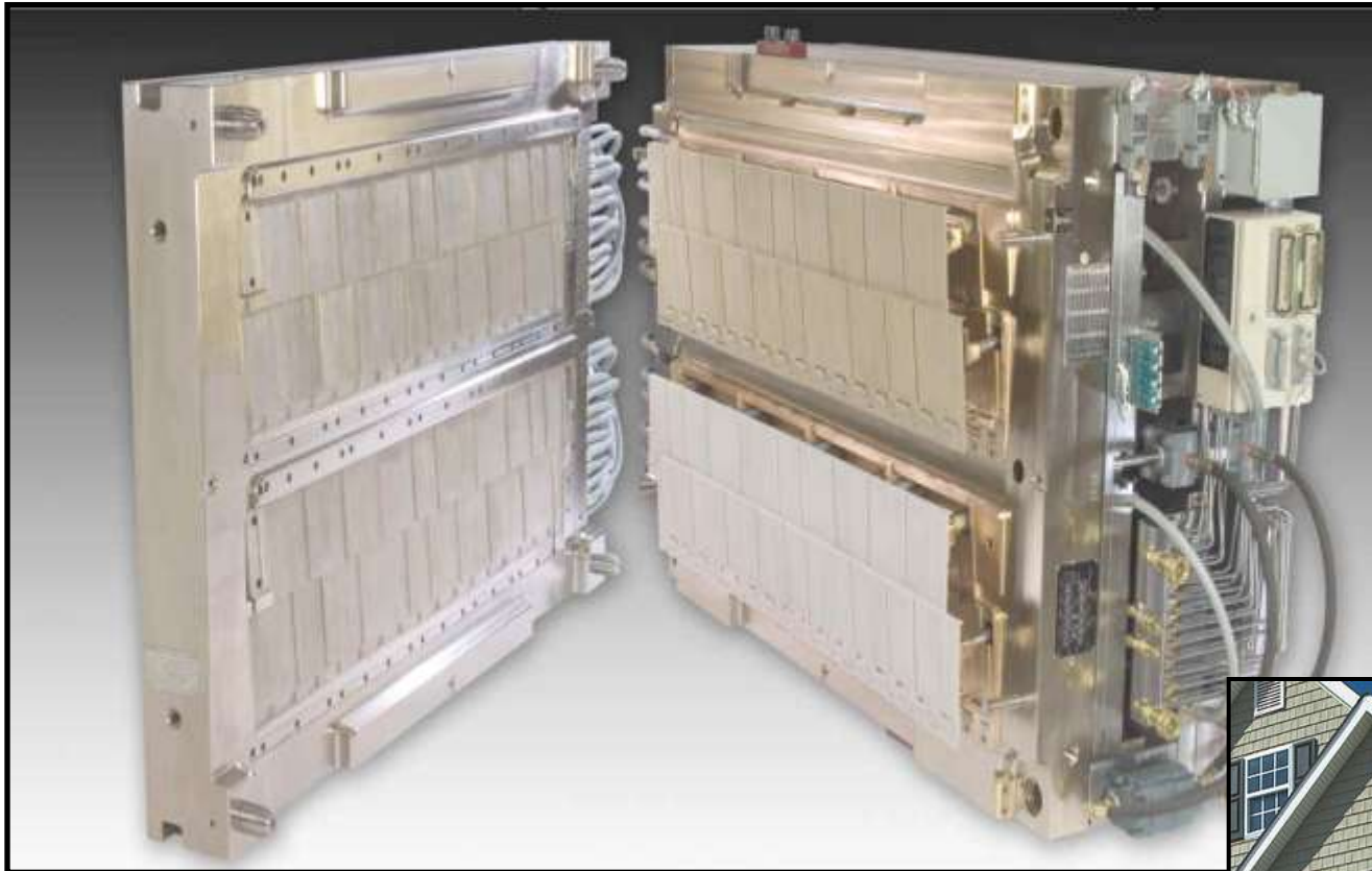
2 CAVITY MOLD FOR RESIDENTIAL ROUGH SAWN SIDING; CUSTOMER NAILITE.
