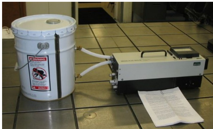
Figure 1. The test set-up used to measure styrene evolution from molded plaques over time with an IR detector.
