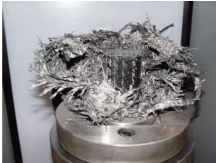
Figure 7 Dynamically compressed carbon fiber composite crush tube showing delamination, corner splitting and matrix damage due to bending.
