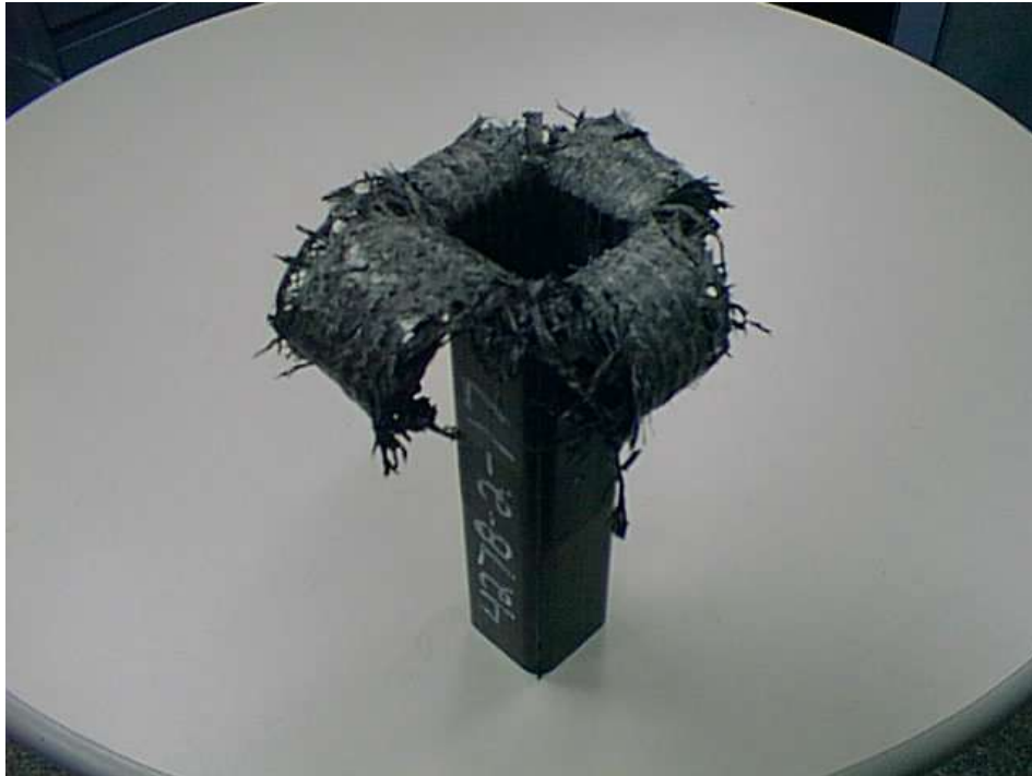
Figure 6 Quasi-statically compressed carbon fiber tube showing delamination, corner splitting and matrix damage due to bending.
