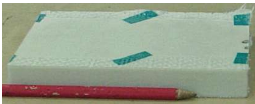
Figure 9: A 2cm thick vacuum infused APA-6 composite.
