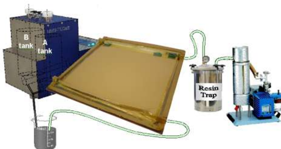
Figure 2: Infusion equipment. Left: Mini Mixing Unit “MMU-TU Delft”, center: bagged fiber lay-up, right: resin trap and vacuum pump with cold trap.
