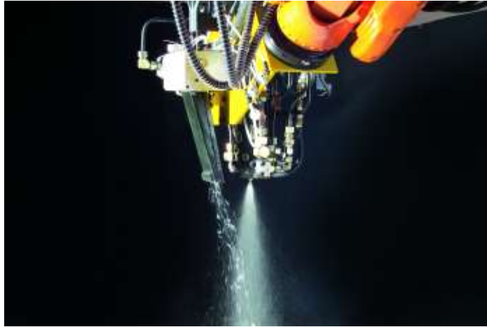
Figure 4: CSM Module Glass Chopper Unit: Wetting on the Fly
