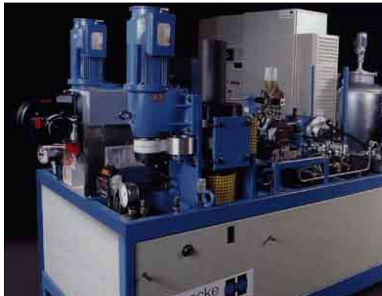
Figure 5: HT Cylinder Metering Module
