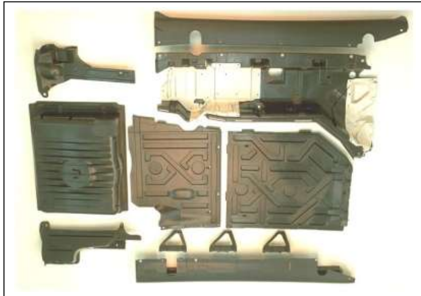
Figure 1: Under-floor system for the 1997 MY Mercedes A Class, showing tunnel with aluminium heat shield (top, 2-color part), 2 large GMT shields (center), rocker panels (top and bottom most – also molded from GMT), and to the left, center, the GMT spare wheel well and 2 small GMT side panels
