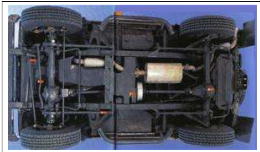
Figure 3: Under-floor system for Range Rover Defender SUV uses no underbody closure system
