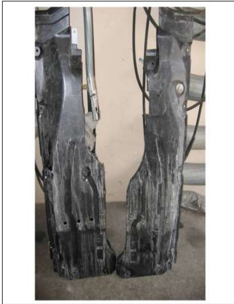
Figure 9: Under-floor panels for the new Mercedes M Class vehicle after driving tests that forced the panels to bear the weight of the entire vehicle
