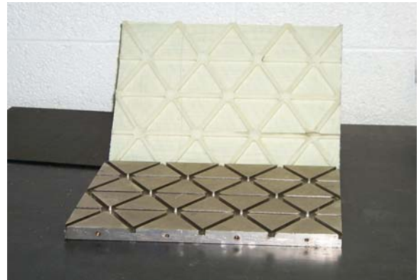
Figure 1. Isogrid panel specimen and mold.
